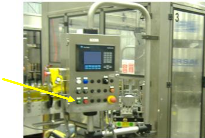
figure 1-3: Try to start the LABELER.
