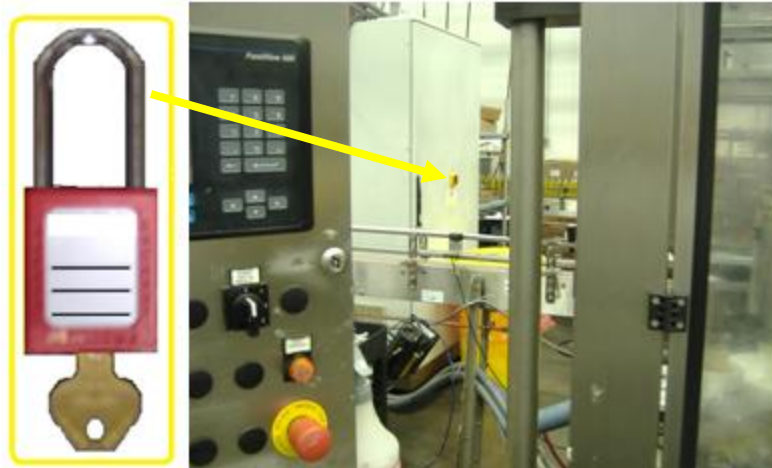
figure 1-4: Lock out MAIN POWER SWITCH.
