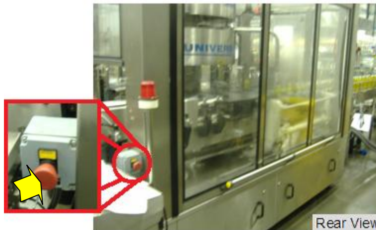
figure 1-2: Location of EMERGENCY STOP PUSHBUTTON.
