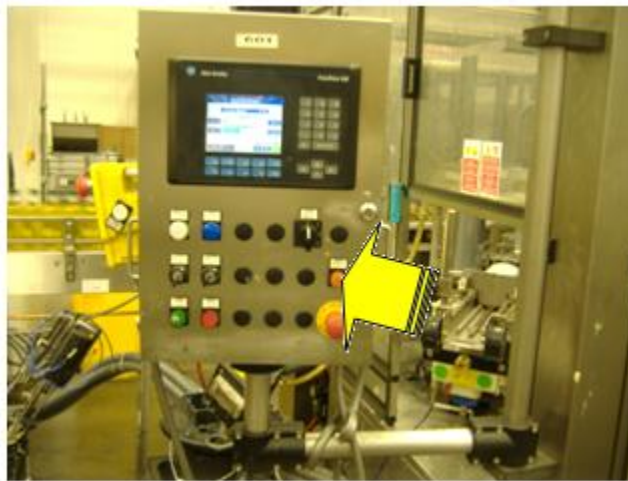
figure 2-2: Press the RESET BUTTON.
