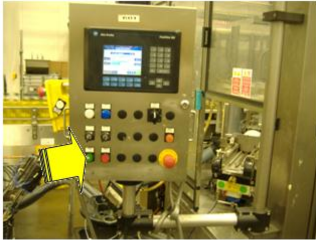
figure 2-3: Press the START BUTTON.
