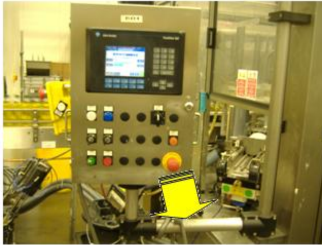
figure 2-1: Pull out the EMERGENCY STOP PUSHBUTTON.
