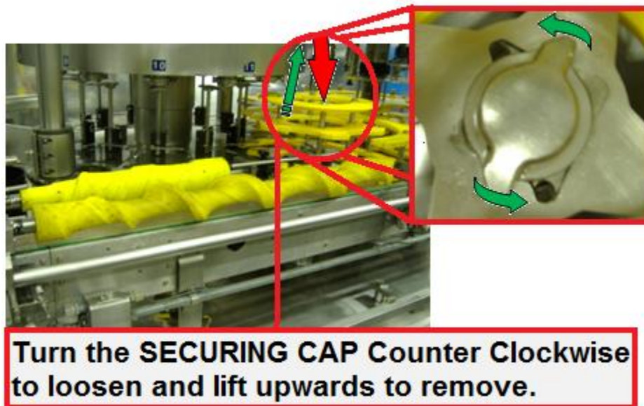
figure 4-2: Removing the INFEED STARWHEEL .
