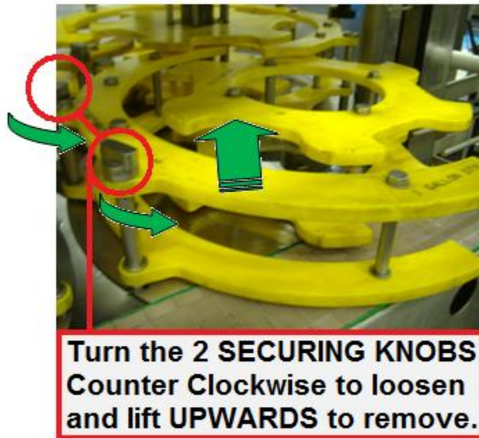
figure 1-1: Removing the DISCHARGE STARWHEEL EXTERNAL GUIDE (#5).
