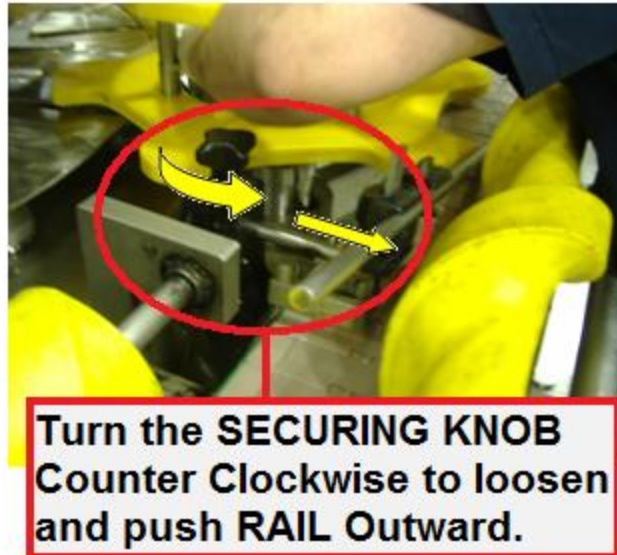
figure 4-1: Loosening the INFEED CONTAINER GUIDE .
